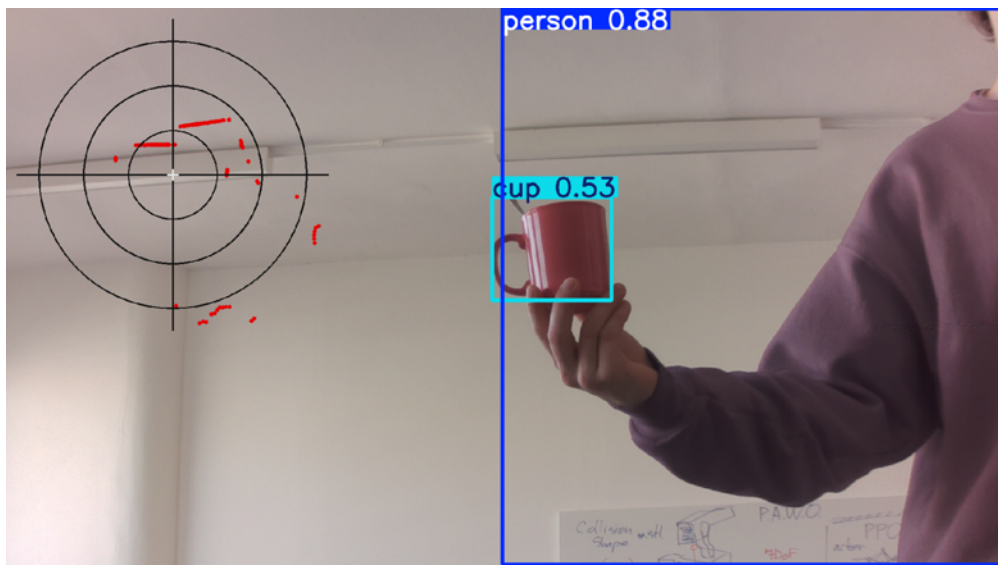
Fig. 3: Visualization of the data available for remote monitoring: 2D LiDAR point cloud (top-left) and the camera's RGB stream with object detection (YOLO) performed locally on Raspberry Pi 5.
