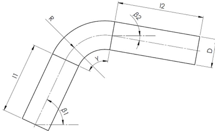
Fig. 1: Controlled parameters of the bent pipe.
