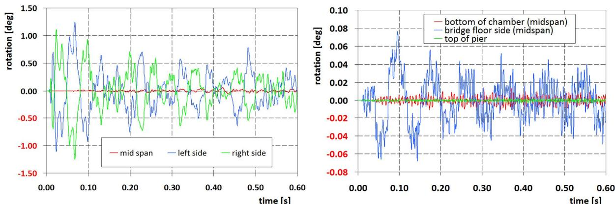
Fig. 4: Time histories of rotations  $F_y$  for above (at left) and under (at right) bridge explosion
