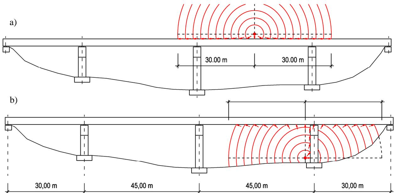
Fig. 2: Location of explosion, a) above the bridge, b) in the vicinity of pier.
