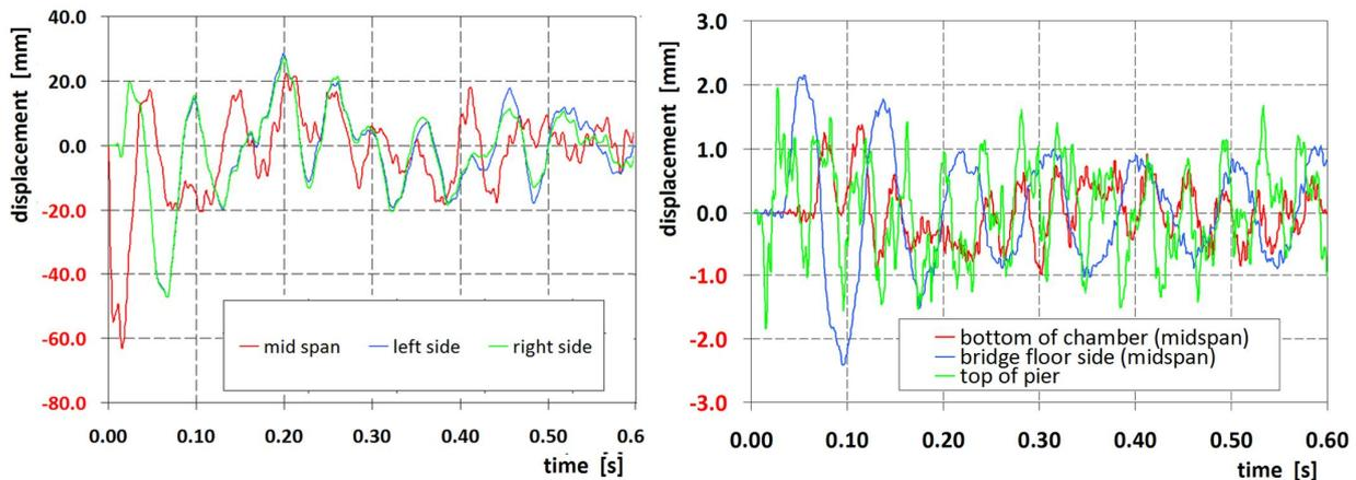
Fig. 3: Time histories of displacements  $U_z$  for above (at left) and under (at right) bridge explosion
