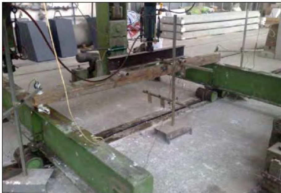
Fig. 3: Test of load bearing capacity in TZÚS Ostrava
