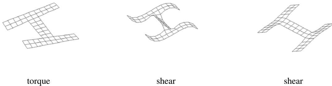
Fig. 2: Example of warping function on I - profile
