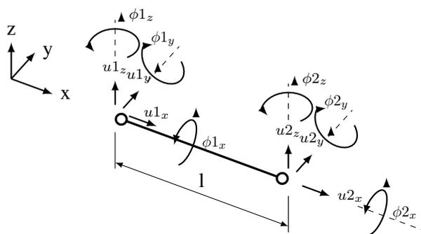
Fig. 1: Beam element
