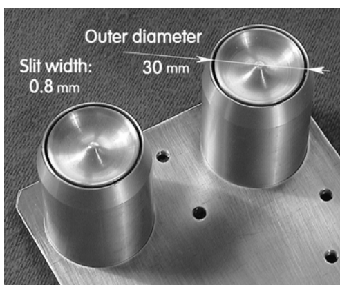
Fig. 6: (Left) The pair of annular nozzles used in the laboratory model. Each nozzle was connected to one of the two outlets of the fluidic valve.
