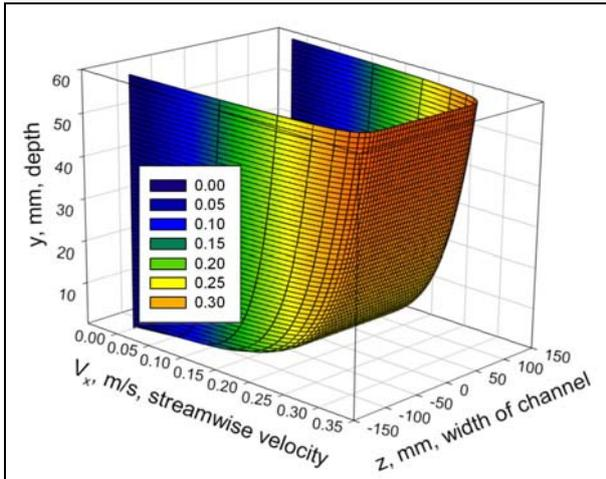
Figure 9. Approximation of the downstream velocity distribution by Eq. (6),  $c = 13.12$ .
