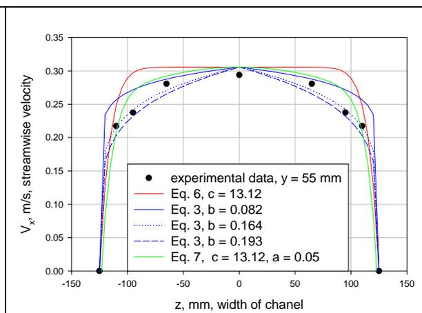
Figure 4. Velocity calculated according to Eqs. (3), (6), and (7).
