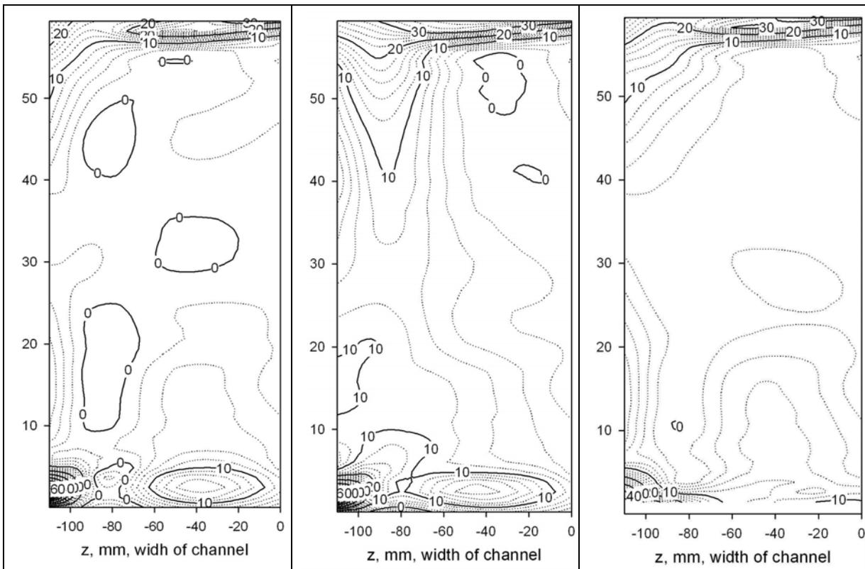
Figure 11. The difference of the experimental and approximated velocity values - left Eq. (3)  $b = 0.082$ ; in the middle Eq. (6),  $c = 13.12$ ; right - Eq. (7),  $c = 13.12$ ,  $a = 0.05$  (in %)
