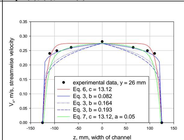
Figure 6. Velocity calculated according to Eqs. (3), (6), and (7).
