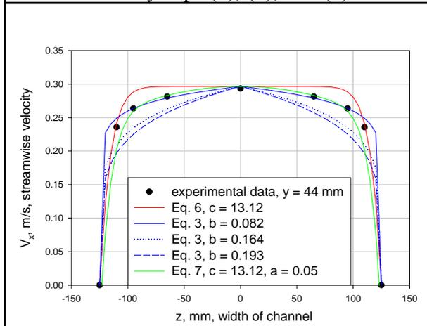
Figure 5. Velocity calculated according to Eqs. (3), (6), and (7).
