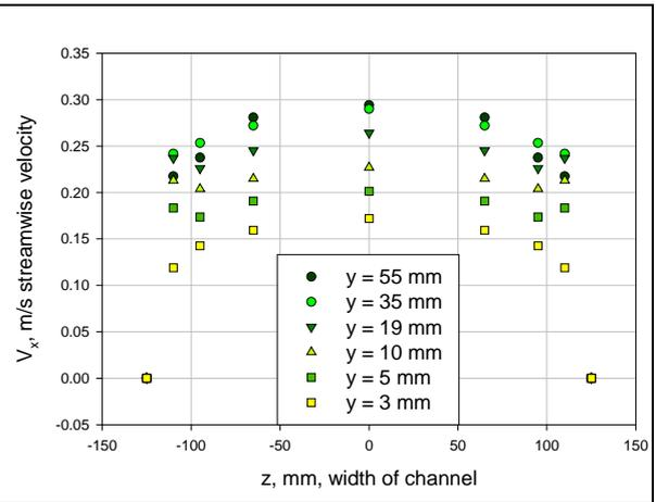
Figure 2. Horizontal velocity profiles at different horizontal planes.
