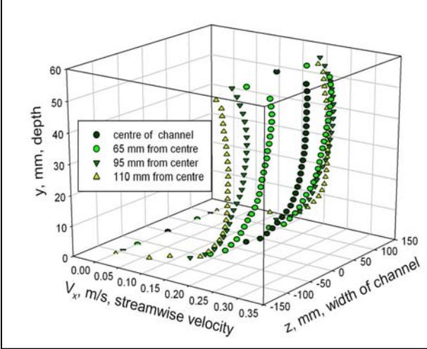
Figure 7. Experimental vertical profiles of the downstream velocity in open channel.
