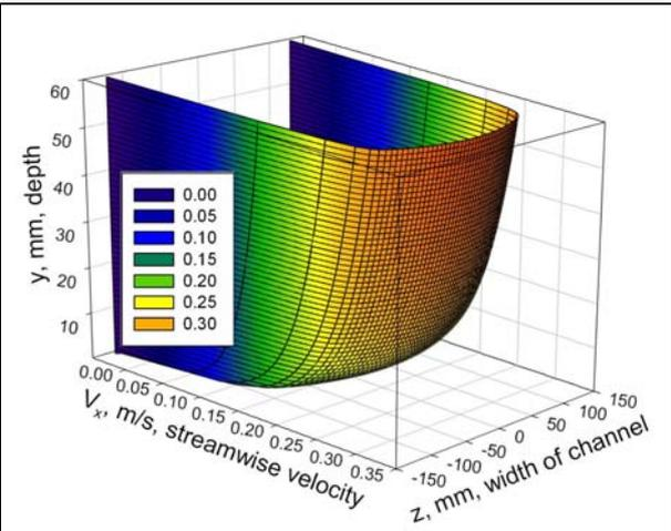
Figure 10. Approximation of the downstream velocity distribution by Eq. (7),  $c = 13.12$ ,  $a = 0.05$ .
