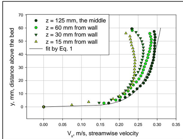
Figure 1. Vertical velocity profiles at different distances from the wall and fit by Eq. (1) with  $u_* = 1.69 \cdot 10^{-2}$  m/s, and  $y_0 = 3.3 \cdot 10^{-5}$  m.
