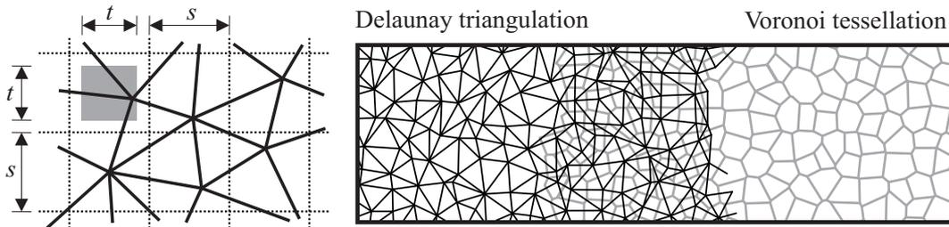
Fig. 1: Left: a generating of the network nodes (according to van Mier (1997)). Right: an example of Delaunay triangulation and Voronoi tessellation of the domain.
