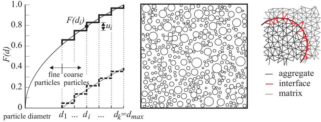
Fig. 2: Left: Fuller curve provides an amount of grains for certain diameters (after Cusatis et al. (2006)); middle: aggregates are placed inside a specimen via random sequential addition; right: three material phases are determined according to node coordinates.
