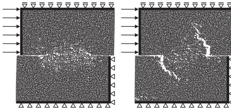
Fig. 7: An ability to simulate the crack pattern for two lattice model types. Left: the truss lattice; right: the rigid-body-spring network.
