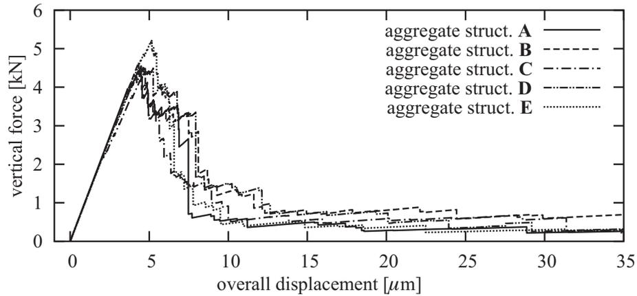
Fig. 11: Responses measured during uniaxial tensile test simulations for various aggregates structures. Amounts of grains and their diameters are identical in all cases.
