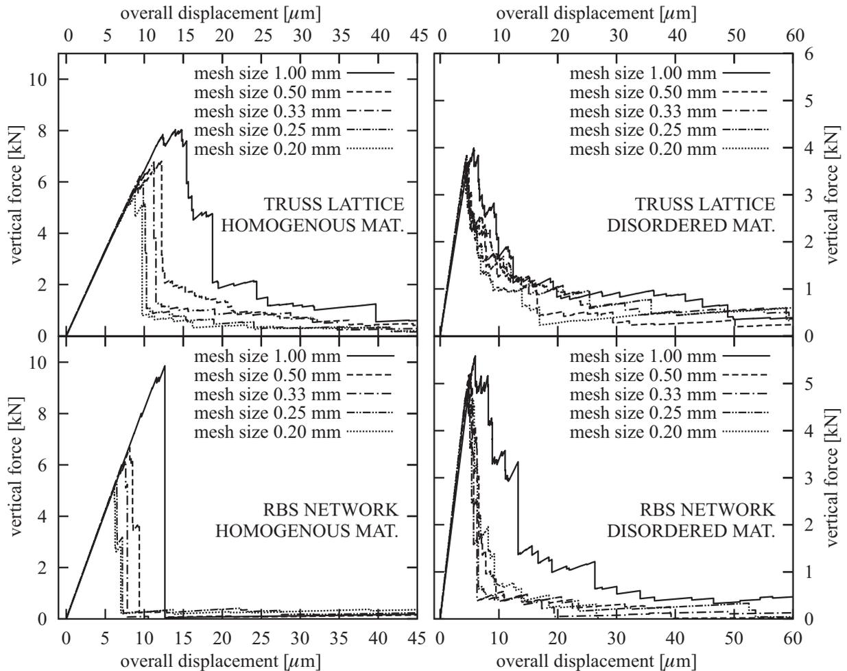
Fig. 9: Responses measured during uniaxial tensile test simulations for various network sizes. The disordered material includes aggregate structure which is identical for all simulations.
