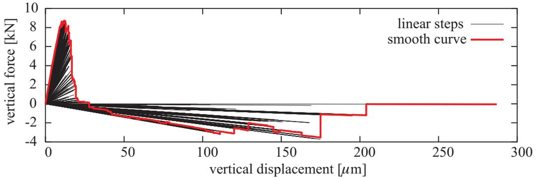
Fig. 5: The response consists of many linear steps. Only steps with increasing prescribed displacement are accepted.
