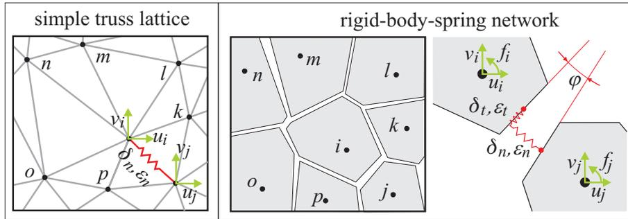
Fig. 3: Nodes of lattice interconnected by springs. Left: the truss lattice, two degrees of freedom per each node; right: the rigid-body-spring network, three degree of freedom per each node.
