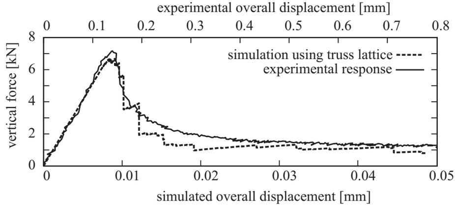
Fig. 6: A record of the uniaxial tensile test and a corresponding simulation using the truss lattice model. A discrepancy between displacements measured during experiment and simulated displacements is probably caused by an incorrect setting of measuring device.
