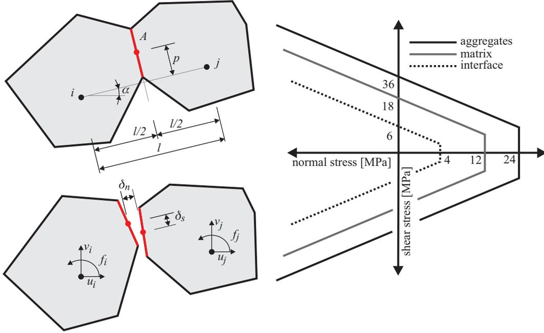
Fig. 4: Left: the motion of rigid bodies, variables description; right: the elemental breaking envelope for different material phases.
