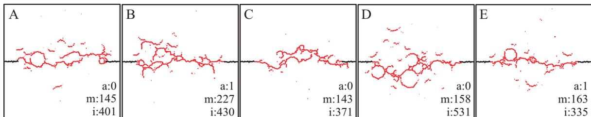
Fig. 12: Crack patterns of virtual specimens subjected to uniaxial tension with variable grain positions. Numbers of cracked elements from each phase are plotted.
