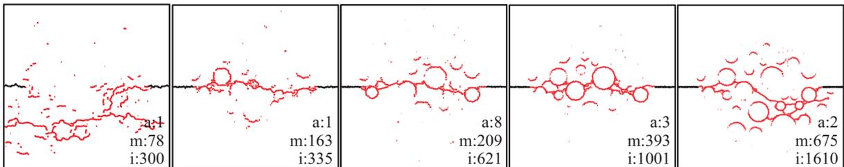
Fig. 10: Crack patterns of virtual specimens subjected to uniaxial tension. Numbers of cracked elements from each phase are plotted.
