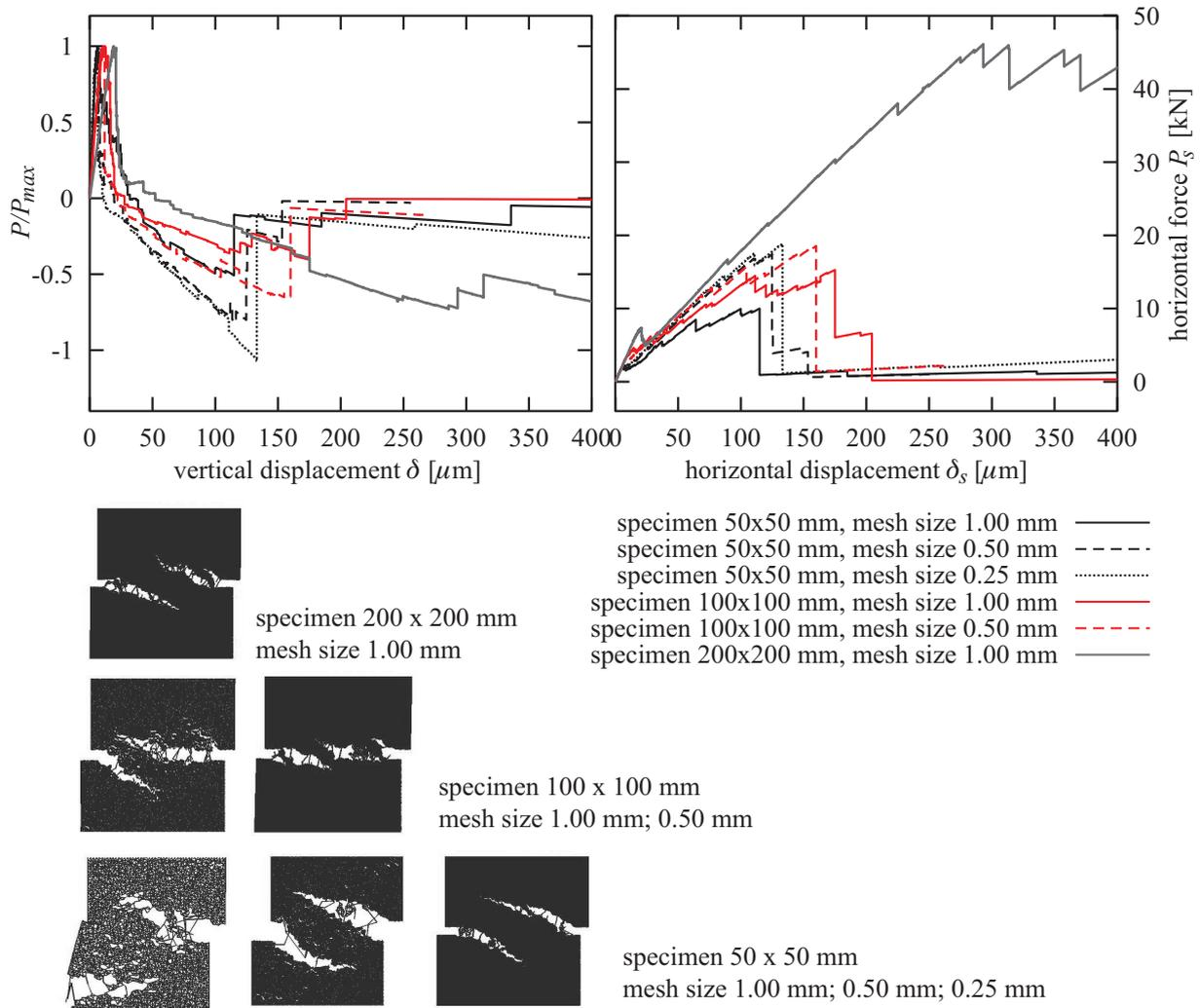
Fig. 8: Responses and crack patterns of virtual specimens subjected to the mixed-mode loading according to Nooru-Mohamed (1992).
