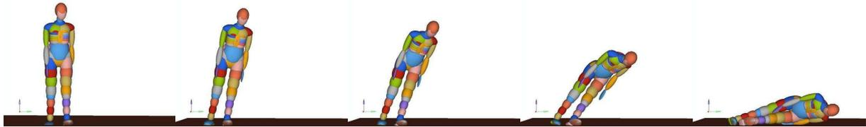
Figure 2: Rigid body reconstruction of the fall using the 5% pedestrian model
