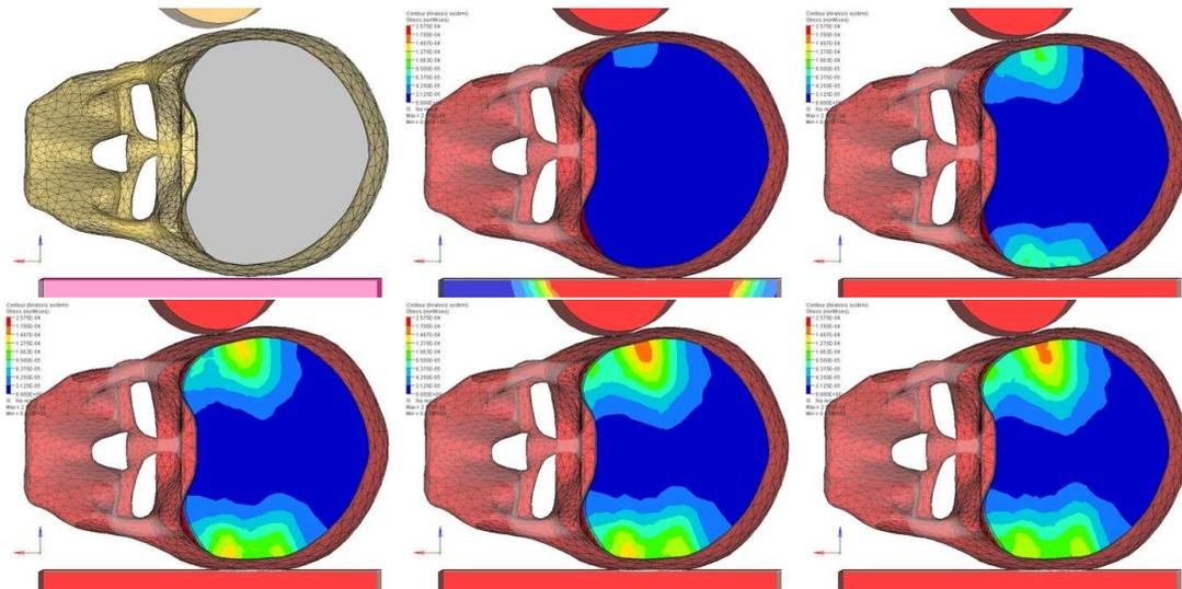
Figure 4: von Mises stress in the brain tissue in 0, 2, 4, 6, 10 ms time intervals
