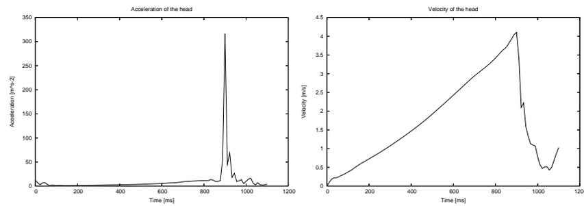
Figure 3: Velocity and acceleration history in the center of gravity of the head
