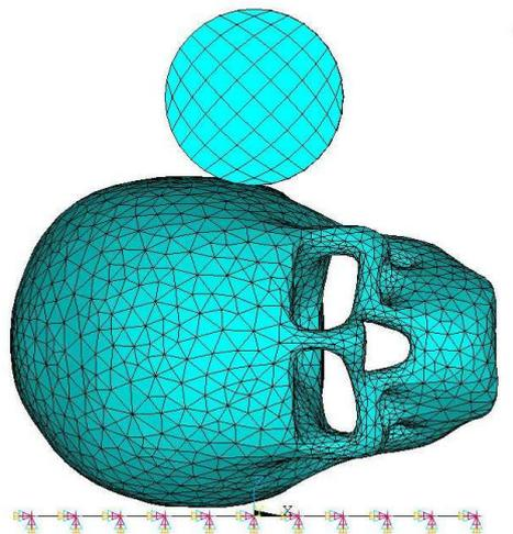
Figure 1: FE model of the skull showing the upper bar of the falling cage
