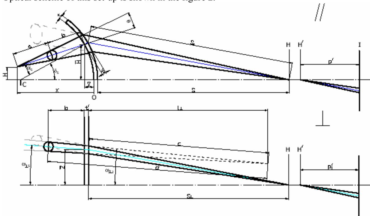
Figure 2 Optical scheme of the devised system with cylindrical tube set-up.
