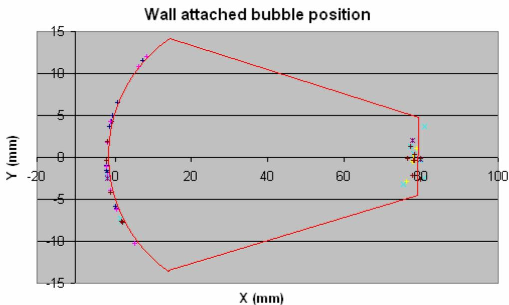
Figure 10 Experimental determined position of chosen wall attached bubbles. Red lines indicate margins of sharply viewed volume.
