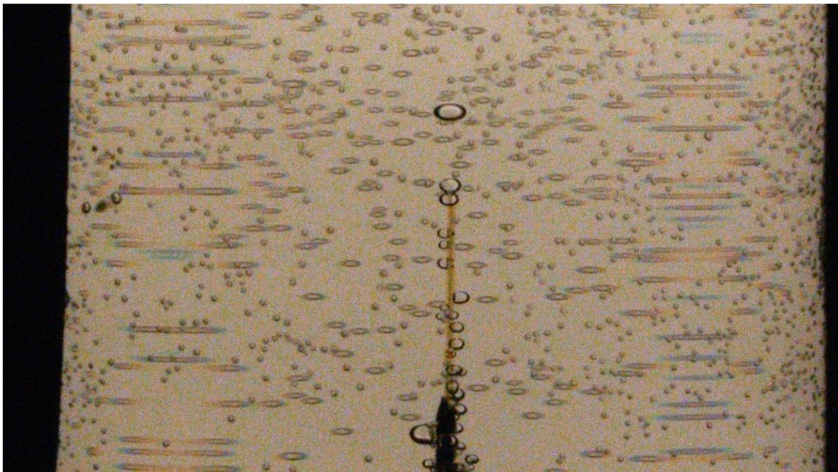
Figure 9 Field of depth in the image is larger than vessel depth equal to 77 mm (much more than glass tube diameter equal to 50,2 mm). Both bubbles attached to the front (circles) and rear (ellipses) glass wall are observed.
