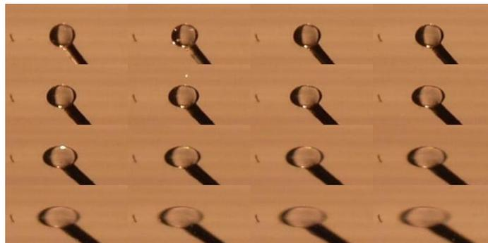
Figure 8 Images of glass sphere inside the cylindrical glass tube filled with water at different axial distances. Axial position difference is 4 mm.
