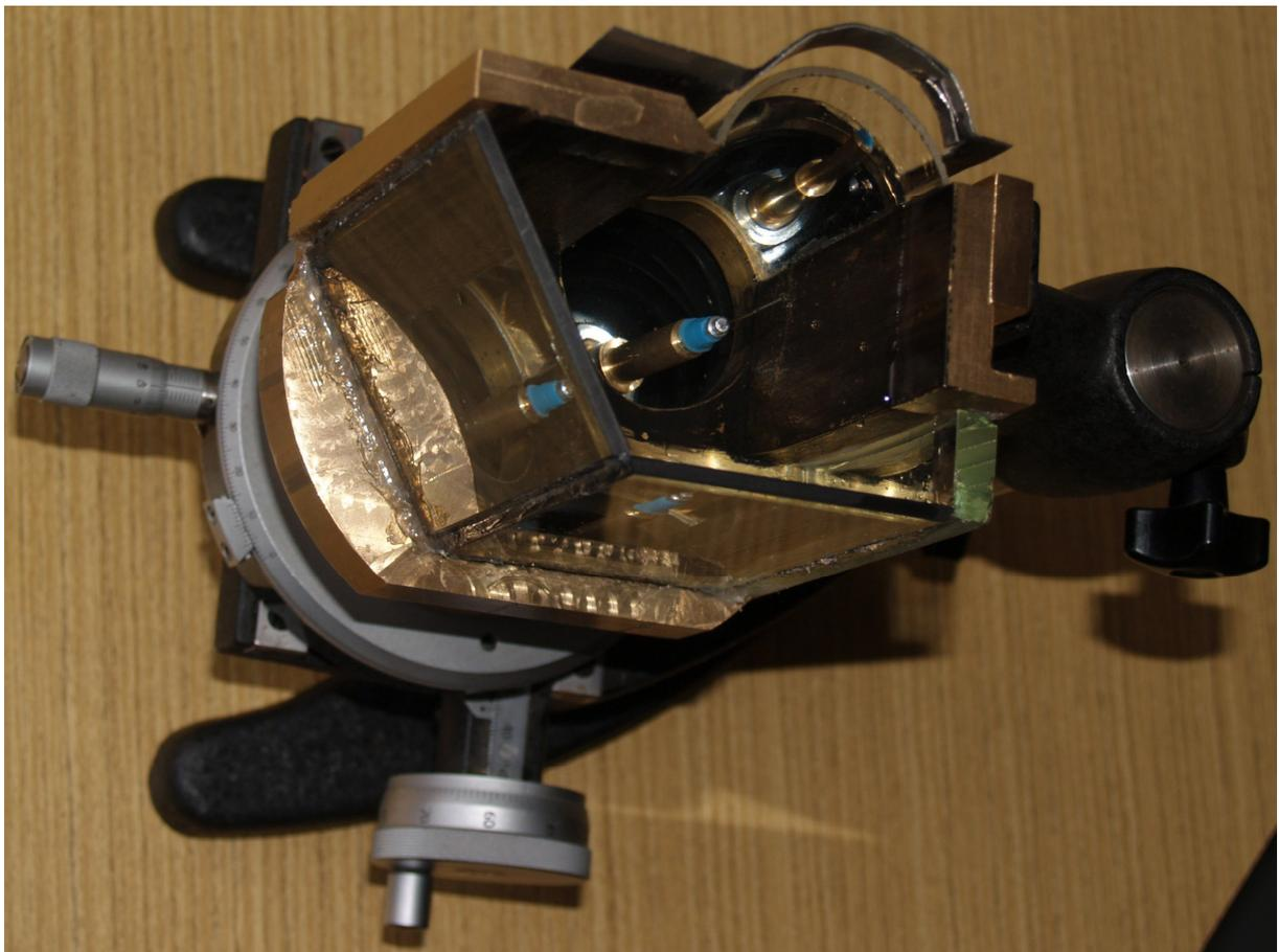
Figure 5 Experimental vessels with XYZ movable support.
