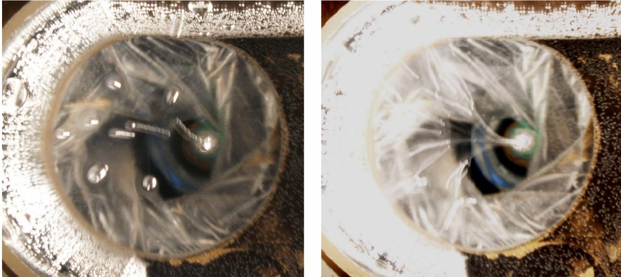
Figure 7 Aerial view on the bubble rising trajectory took with exposition times  $1/15$  s – left and 1 s right.
