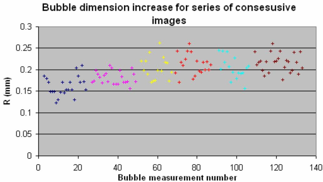
Figure 11 Dimensions of chosen wall attached bubbles of series six consecutive images.
